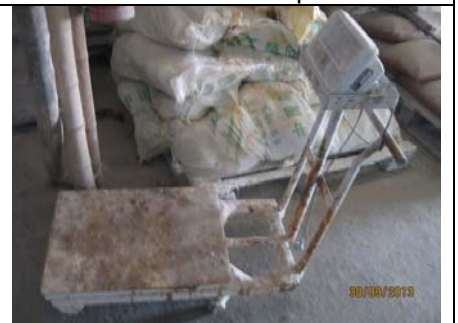
(21) Electronic balance not calibrated in raw materials warehouse
