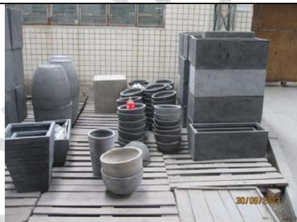
(20) Non-conforming semi-finished products not properly identified and segregated in semi-finished products warehouse
